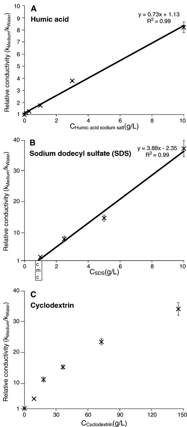
**FIGURE 4.** Diffusive flux increased at increasing concentrations of (A) humic acids, (B) sodium dodecyl sulfate (SDS), and (C) cyclodextrin; cmc refers to the critical micelle concentration. Linear regression is included in Figure A and B.
