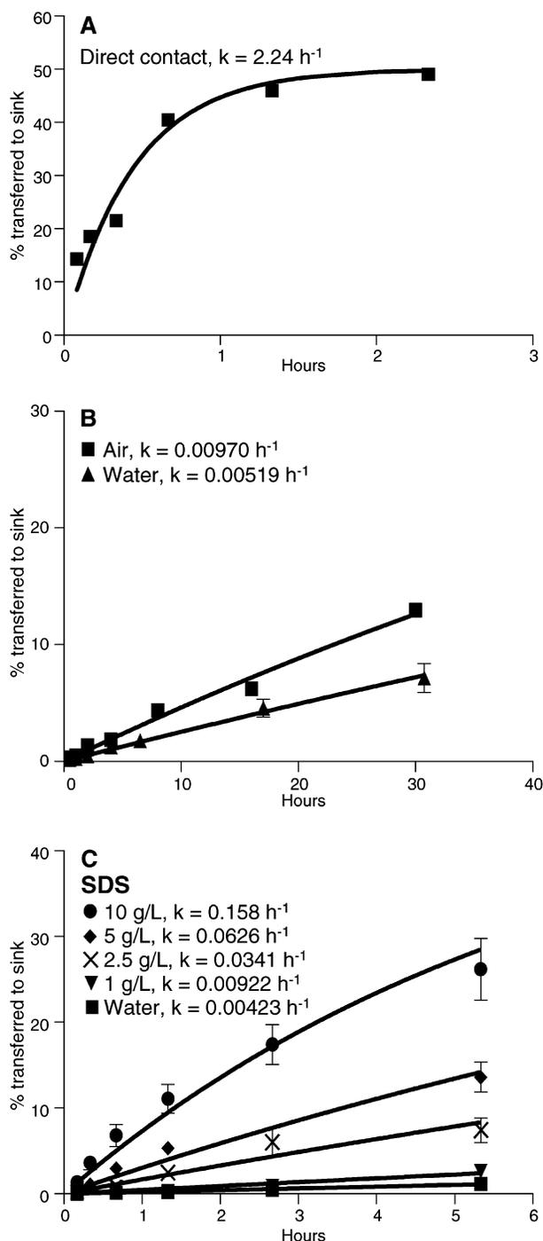
**FIGURE 3.** (a) Within about 1 h fluoranthene was evenly distributed between source and sink (direct contact), (b) whereas the presence of an aqueous or gaseous UBL prolonged equilibration times by orders of magnitude. (c) The diffusive flux increased at increasing concentrations of the surfactant SDS. Standard deviations between replicates are included as error bars, which in some cases are smaller than the symbols. Least-squares fits to eq 6 are included as solid lines.
