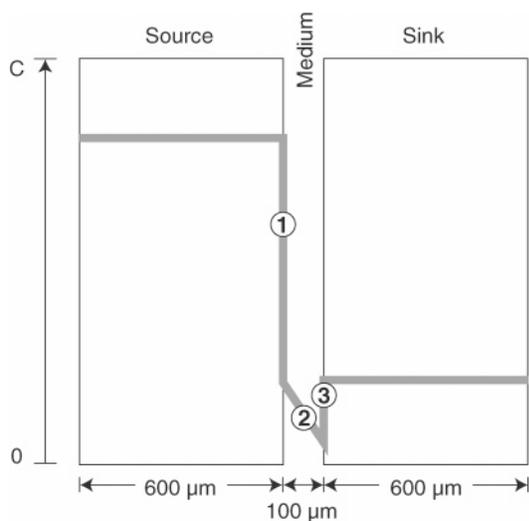
**FIGURE 2.** Concentration profile within the experimental apparatus including the three steps that are involved in the mass transfer from source to sink: (1) partitioning,  $C_{\text{Medium}} = C_{\text{Source}}/K_{\text{PDMS,Medium}}$ ; (2) diffusion, flux =  $-D \times \Delta C/\Delta x$ ; and (3) partitioning,  $C_{\text{Medium}} = C_{\text{Sink}}/K_{\text{PDMS,Medium}}$ .
