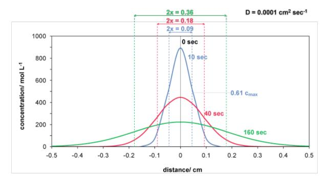
Equation 3 also allows to estimate characteristic values for the situation in Figure 1. When entering the thickness of the film for x in equation 3 then a time t can be calculated. This time t is close to the time that is needed for equilibration of the film with the outside through the diffusion process. Within this time t roughly 3/4 of the final number of molecules has diffused into the film.
